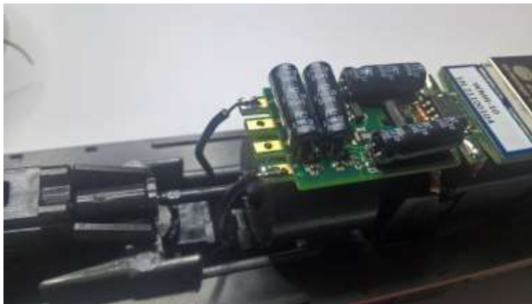
Figure 14 Solder the wires from the rear truck.
