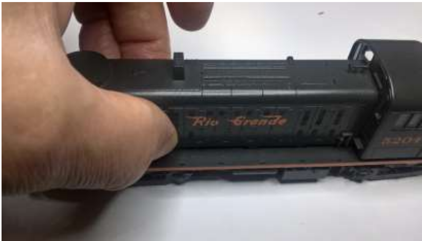
Figure 2 Removing the locomotive body
