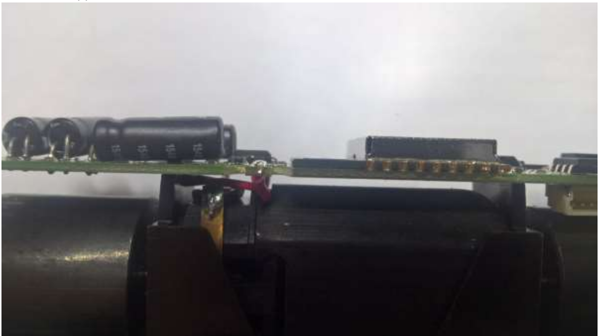
14. Figure 12 Look underneath the WMR-10 unit to make sure the wires do not touch any other part.
