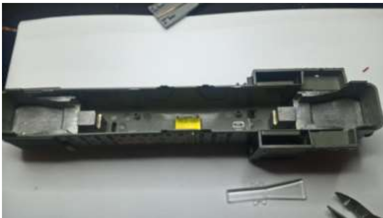
Figure 22 The body shell with the cut light guides and weights in place.
