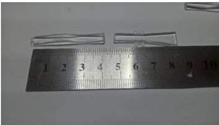
Figure 19 Cut the front light guide to 40mm.
