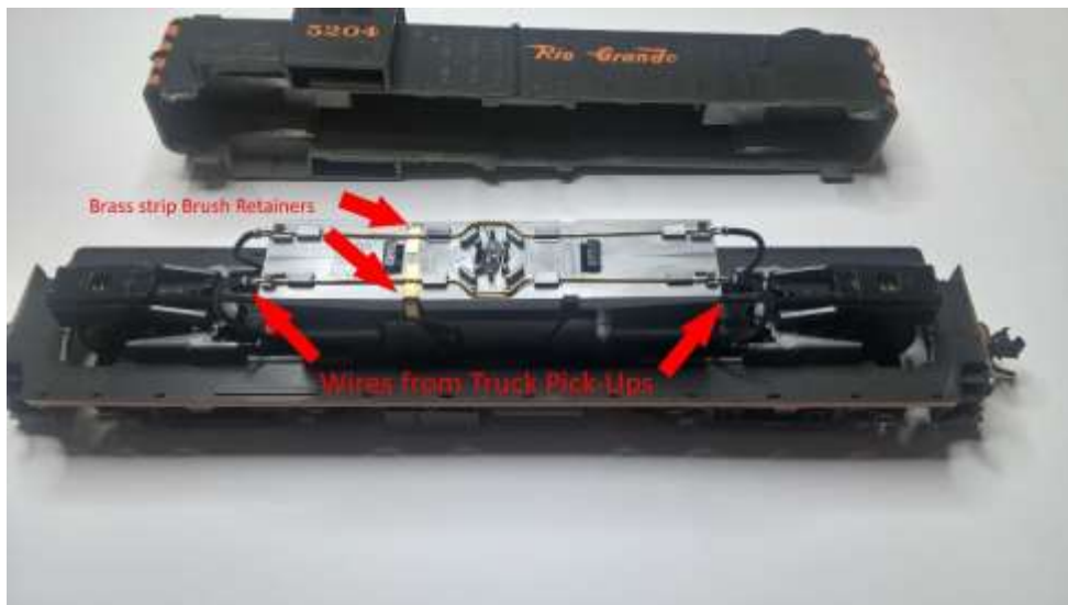
Figure 3 Original internal construction of the Atlas/Kato (Japan) RS3
