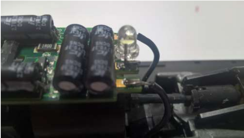
Figure 17 LED soldered in place for the front light.
