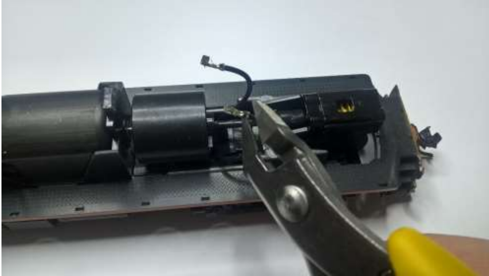
Figure 7 Cutting the clips from the pick-up wires.
