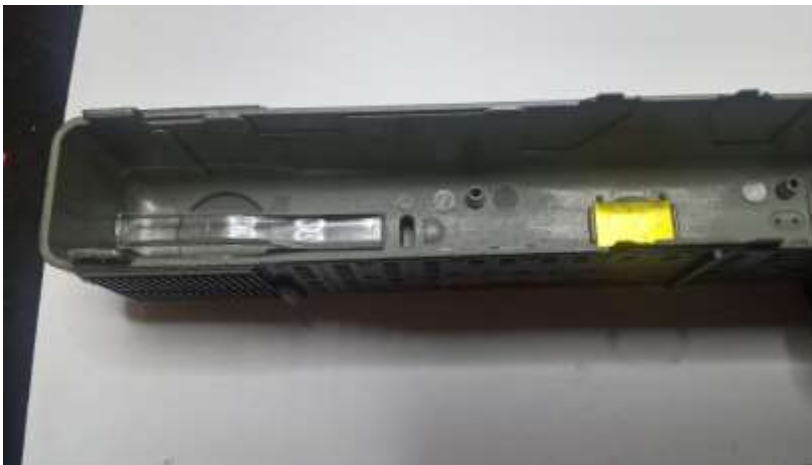
Figure 21 The cut rear light guide in place.
