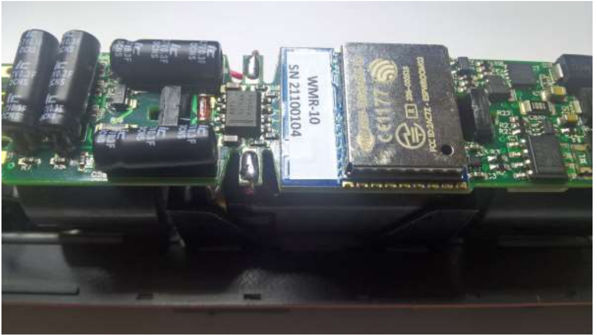
Figure 11 The wires from the brush retainers soldered to the WMR-10 side tabs.
