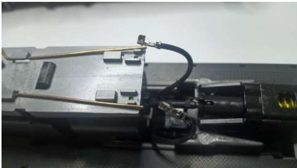
Figure 4 Removing the pick-up wires from the lamp retainer
