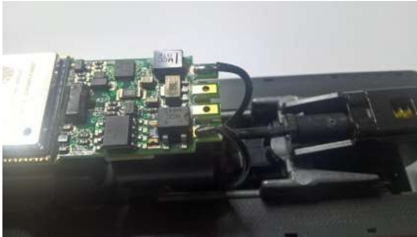
Figure 13 Solder the wires from the front truck.
