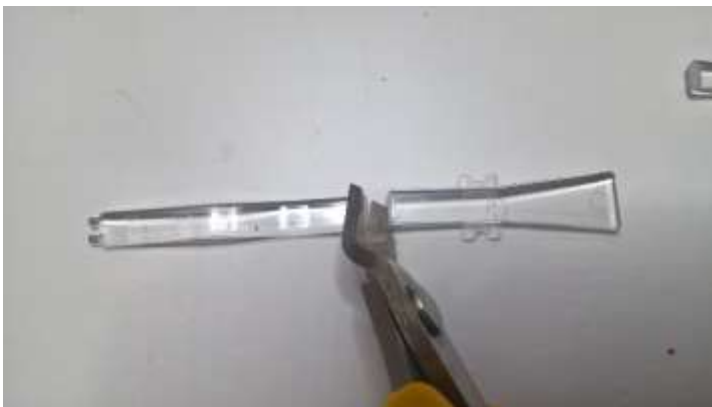
Figure 18 Cutting the light guides from the original locomotive.
