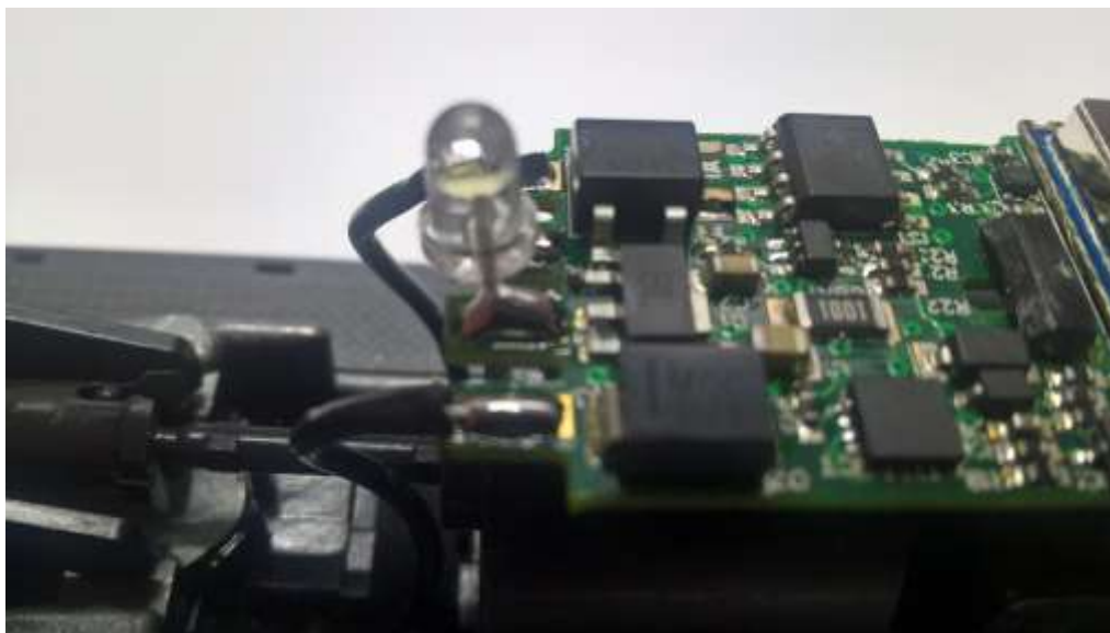
Figure 16 LED soldered in place for the rear light.
