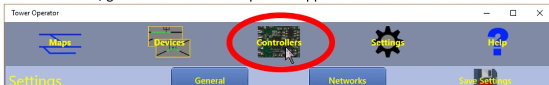
The Controllers screen allows you to scan the operating network for WifiTrax controllers. Since you have set the operating network to the WUFP-40's own private network, there will only be one IP address to scan and one controller visible. Click the Scan button
