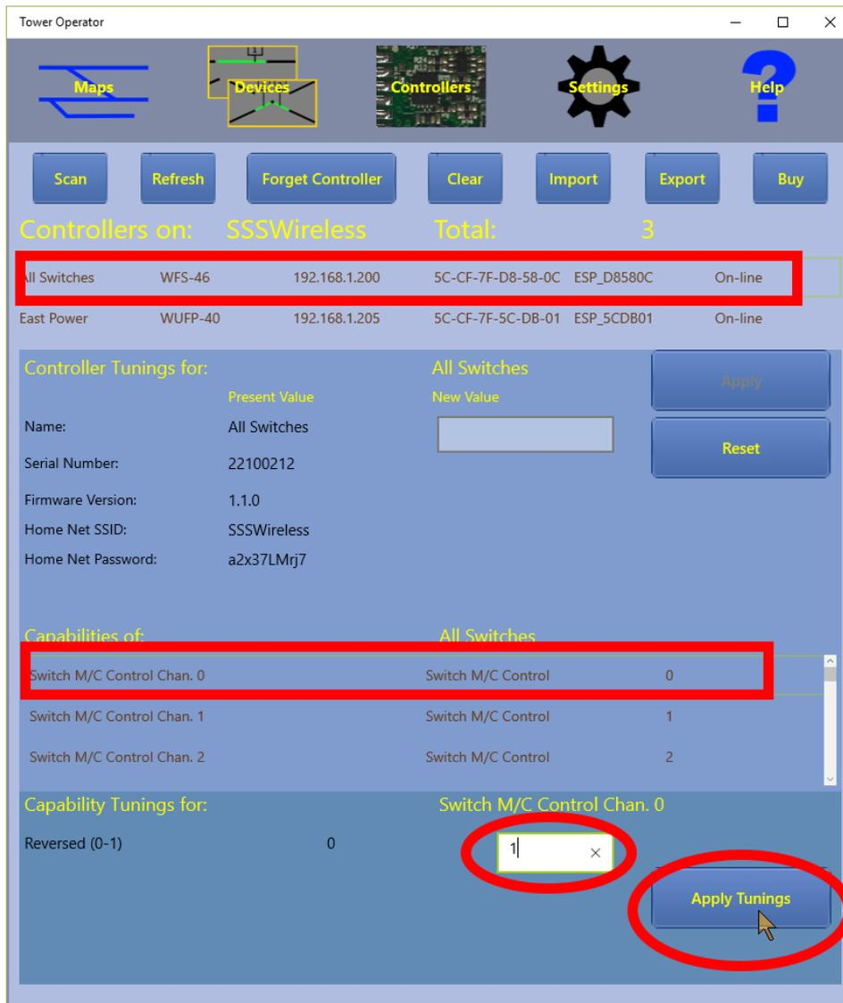
Figure 41 Changing the "Reversed" Tuning Value for an Incorrectly Wired Switch
