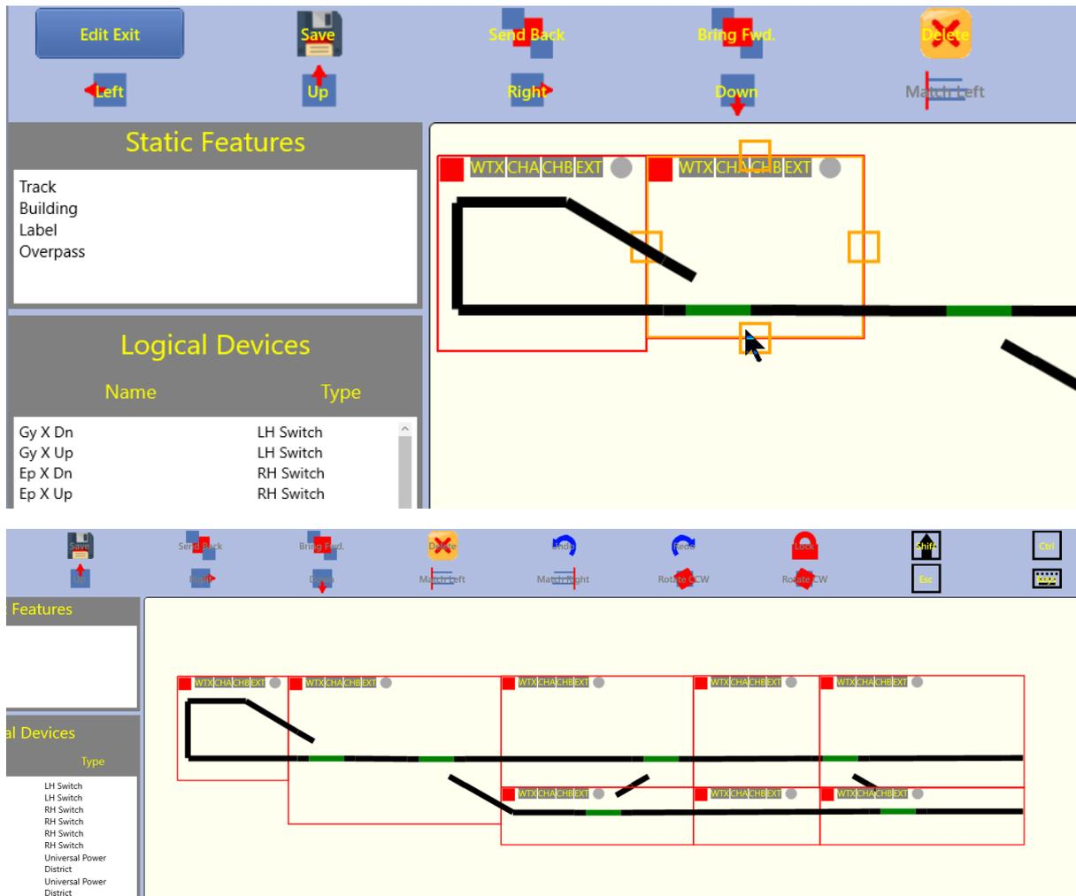
Figure 36 All the Switches, Track and Power Blocks are Complete
