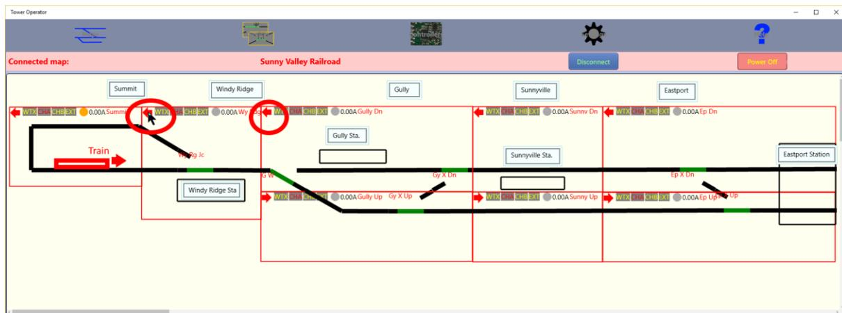
Figure 52 Correct the Switch Settings and Reverse the Windy Ridge and Gully Dn Blocks
