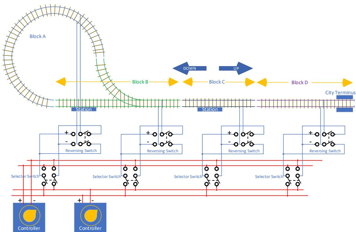
Figure 2 A Part of a Model Railroad with a more Complicated Block System
