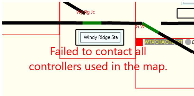
Figure 40 Warning Message when one of the Controllers Cannot be Reached
