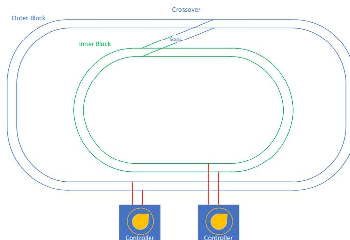
Figure 1 Simplest Block Concept for a Model Railroad
