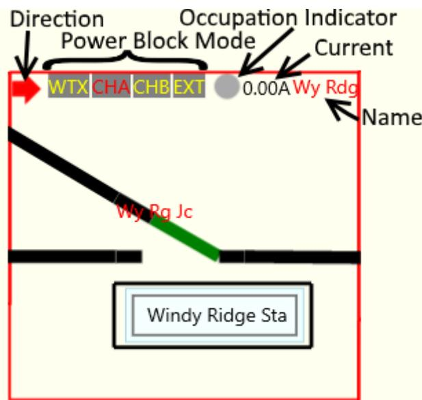
Figure 42 Appearance of a Power Block on a Map
