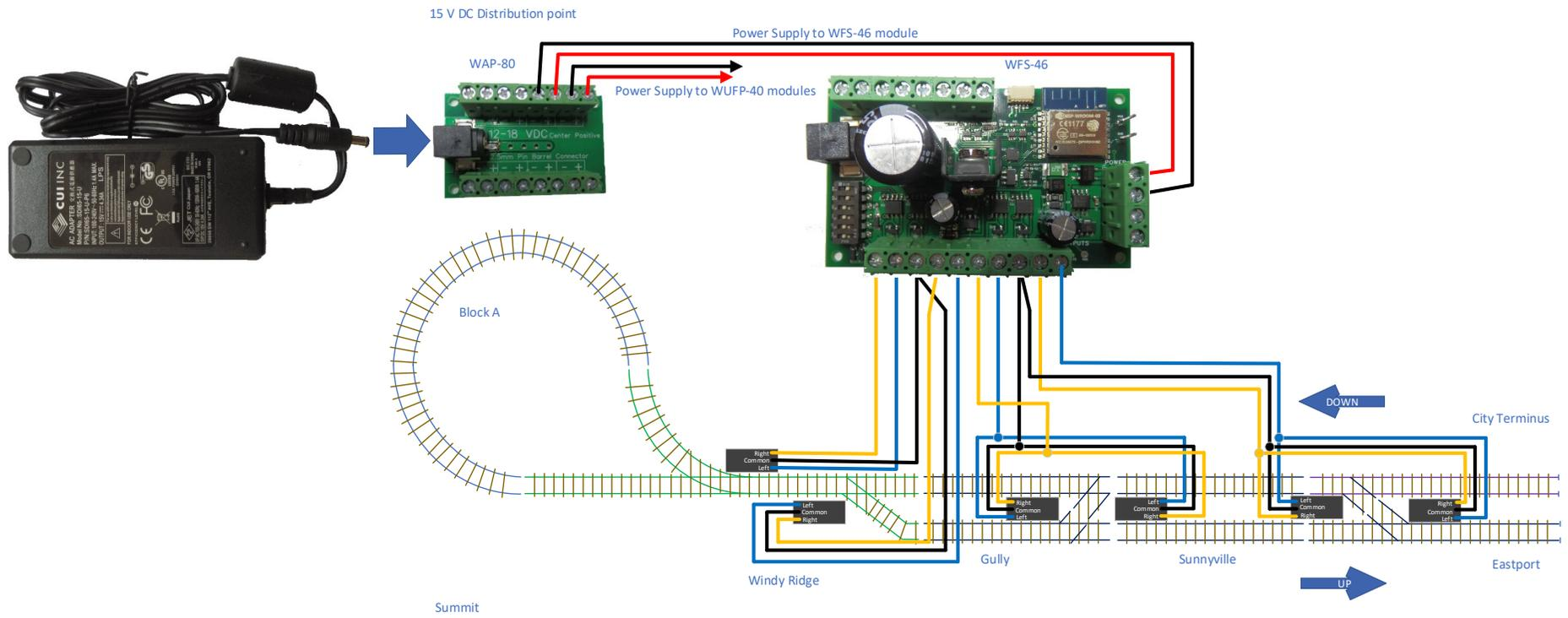
Figure 7 Switch Machine Wiring using the WFS-46
