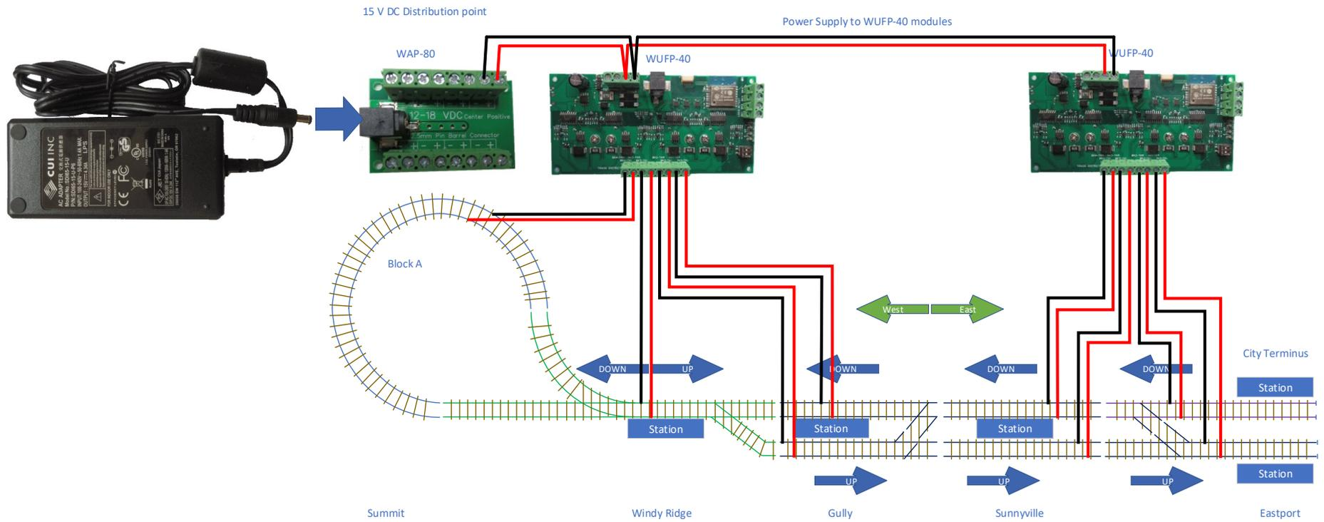
Figure 6 Power Wiring of the Sunny Valley DC Layout
