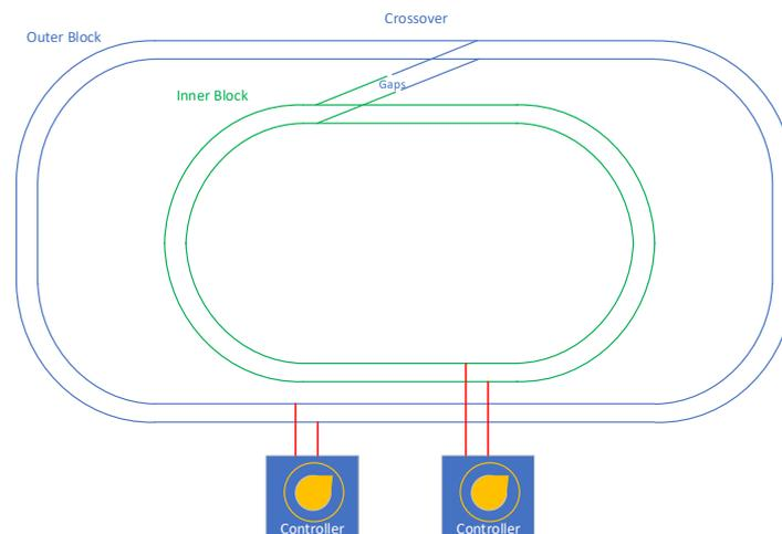
Figure 1 Simplest Block Concept for a Model Railroad
