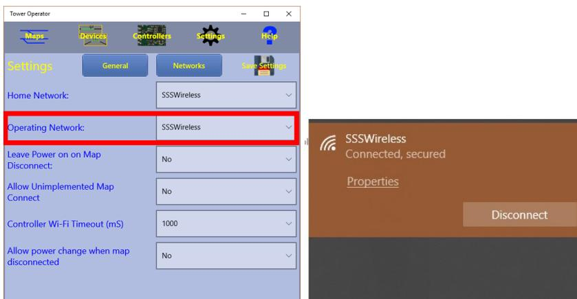
Figure 15 Returning to Operate on the Home Network
