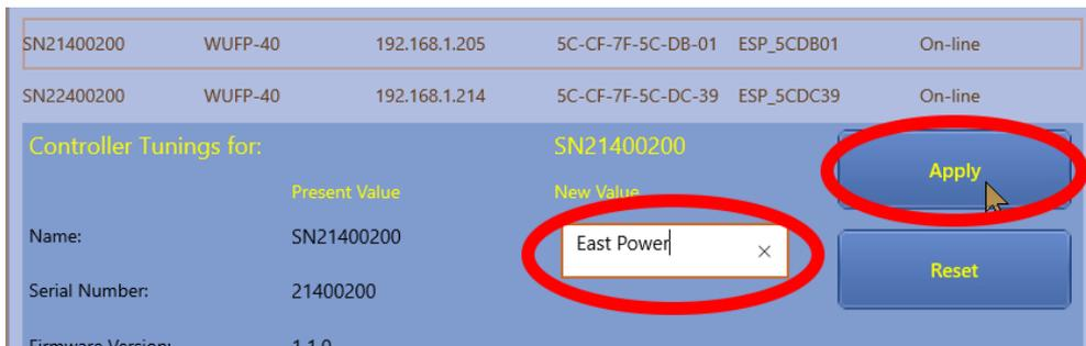
Figure 17 Changing the Name of a Controller
