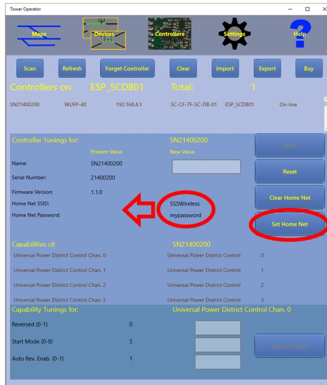
Figure 13 The WUFP-40 Controller Present on its own ESP\_5CDB01 Network. Transfer the Home Network Information to this Controller.
