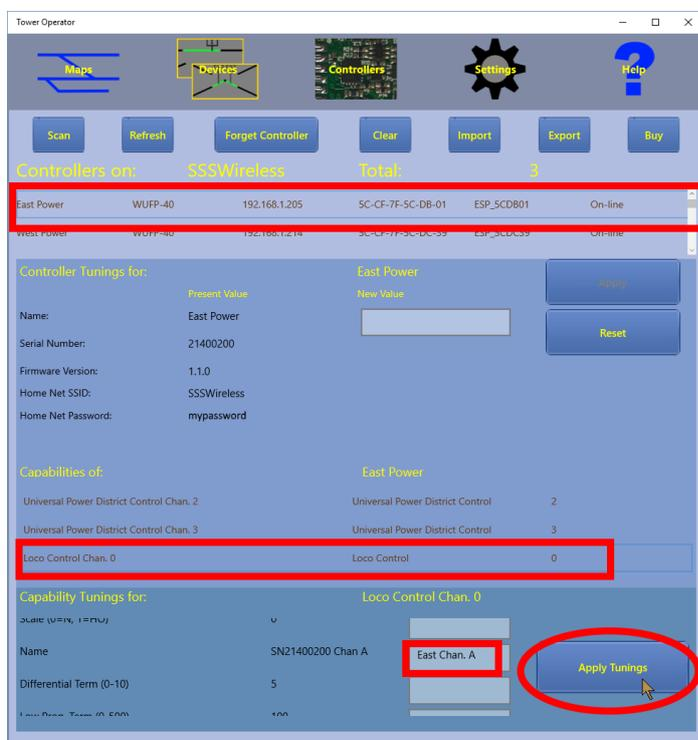
Figure 43 Set the Name of the Loco Control Channels
