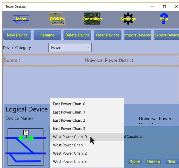
Figure 29 Select the Correct Physical Capability for the Summit Block
