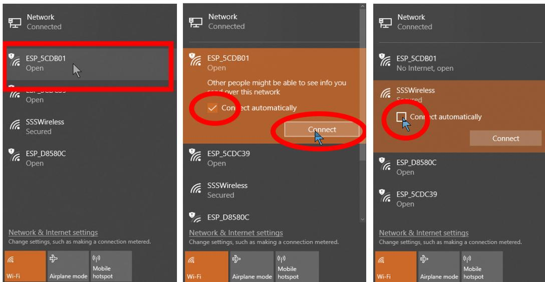
Figure 12 Connecting your Windows 10 Computer to the Controller Network ESP\_5CDB01
