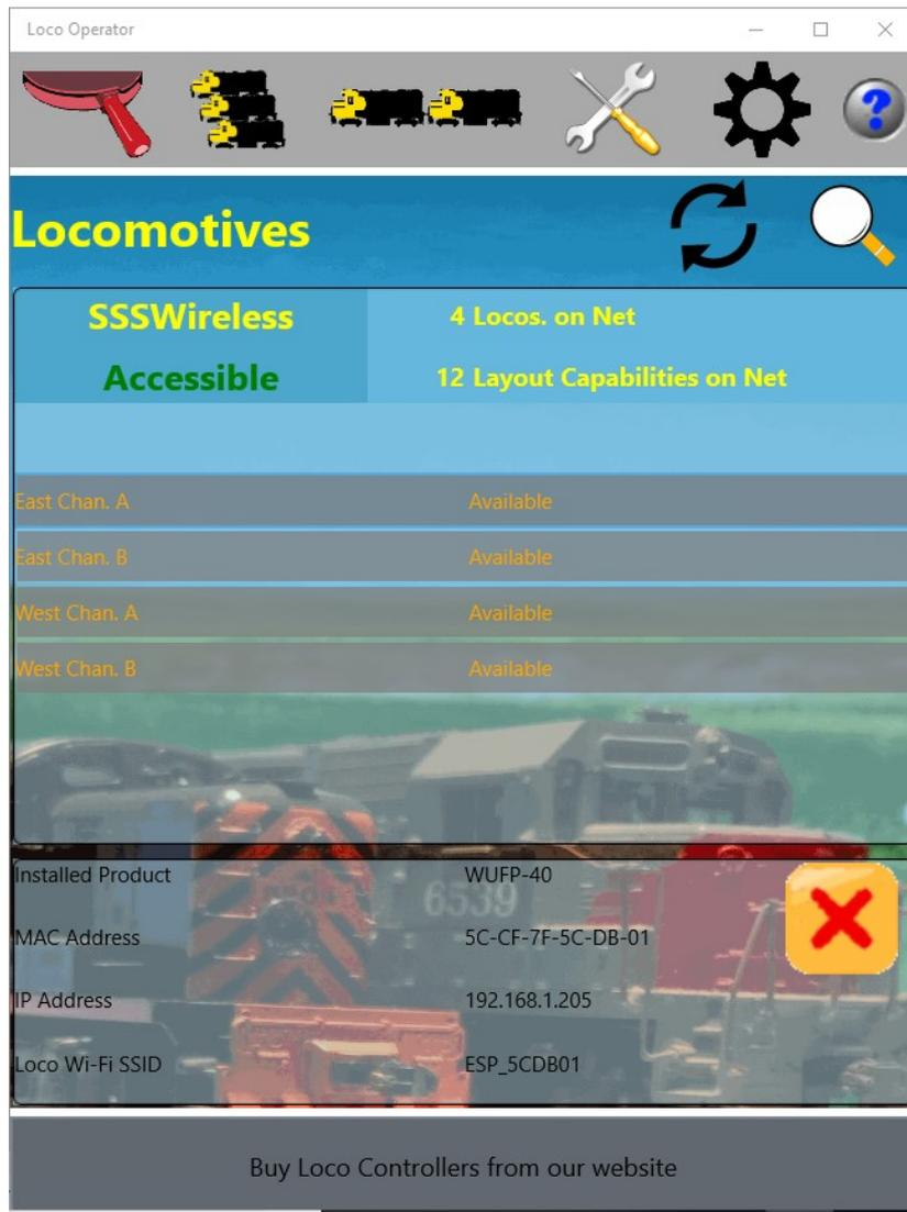
Figure 44 Loco Operator has Found Four "Locomotives" - Really Loco Control Channels on the two WUFP-40 Modules
