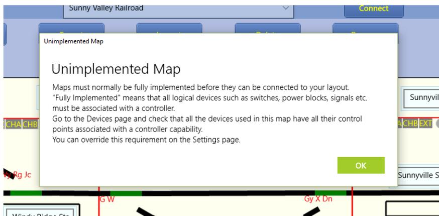
Figure 38 The Unimplemented Map Warning Displays if one or more Logical Devices on the Map do not have a Controller Capability Assigned to them
