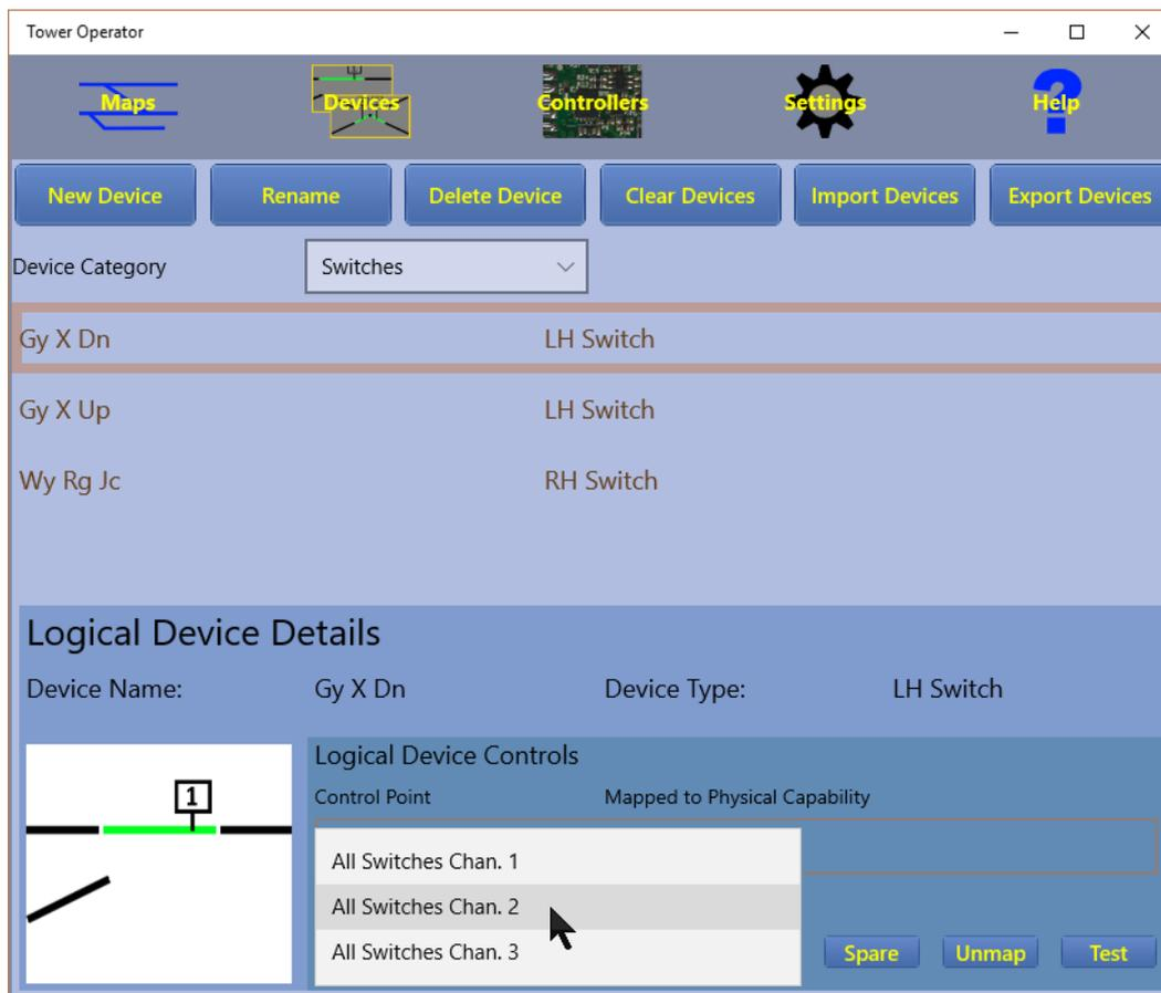
Figure 24 Assigning the Controller Capability for the LH Switch "Gy X Dn"
