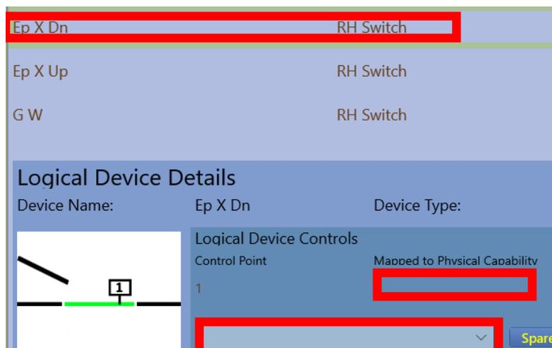
Figure 39 Here a Switch “Ep X Dn” has not been Assigned a Physical Capability on a Controller
