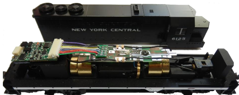
Figure 2 Typical WMH-20 Installation Always put a piece of electrical tape underneath!
