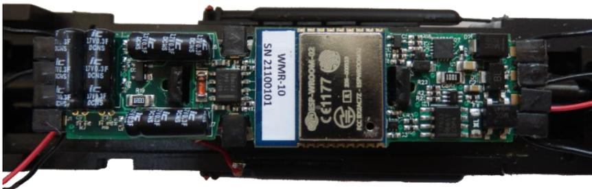
(1) Figure 3 WMR-10 Installed in a locomotive. Here the wires have been attached using the original plastic clips.
