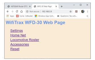
Figure 97 Use the IP Address to open the main menu web page
