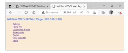
Figure 35 The WFD-30 Main Menu Opened from the Find Modules Tool
