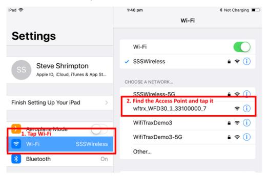
Figure 5 Connecting to the WFD-30 Wi-Fi Access Point
