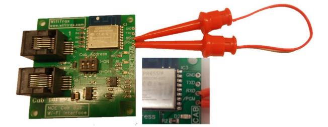
Figure 29 Link attached to force module into Wi-Fi Channel Select Mode on power-up
