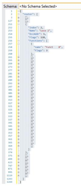
Figure 51 A Loco entry in a JSON Roster File
