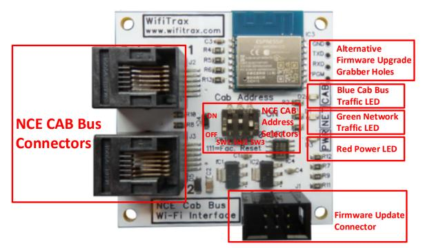
Figure 1 Connections and switches on the WFD-30.
