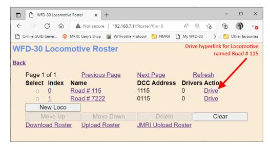
Figure 41 The Drive Hyperlink in the Locomotive Roster Page. Click this to drive the loco.
