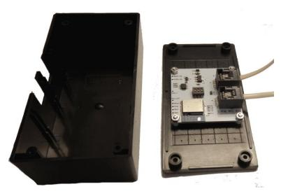
Figure 92 Suggestion for mounting inside a plastic box.
