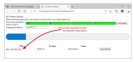
Figure 34 The FindModules Tool has Found your WFD-30 module. Click on the URL to open the Main Menu.
