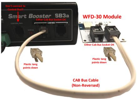
Figure 2 Connecting the WFD-30 Module to your NCE Command Station
