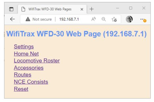
Figure 27 The WFD-30 Web Setup Main Menu
