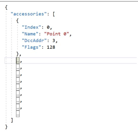
Figure 66 Accessory Entry in a JSON Accessory List File
