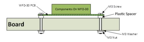
Figure 90 Mounting the WFD-30 on a board
