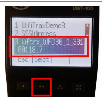
Figure 24 Select the Wi-Fi Network of the WFD-30
