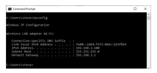
Figure 93 Using ipconfig to find your computer's ip address and default gateway
