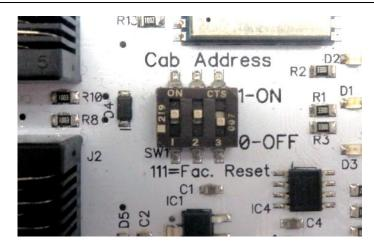
Figure 89 The DIP Switches in default position. Cab bus address 10 selected.
